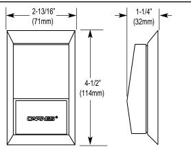
The wall mounted HXHCG Humidistat uses a monolithic sensor and electronic circuitry to provide accurate and reliable humidity sensing. Set point range is 0 to 100% R. H. to cover most application requirements. The HXHCG has a concealed setpoint adjustment with a locking cover to prevent tampering. Ambient operating conditions are from 0° to 85°C.
