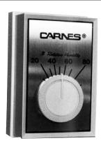
This attractive wall mounted humidistat is a convenient control for mounting in the conditioned space. Select a location four or five feet above the floor in freely circulating air of the temperature and humidity about average for the entire space to be controlled. Avoid locations near hot or cold air ducts and discharge air from the humidifier. Scale range is from 10%-90% R. H. Differential is 5% non-adjustable.
