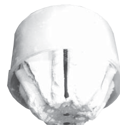
Cut-away used steam cylinder showing mineral deposits.
