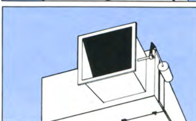
THV3B and THV4B Single Duct Mechanical Reset Constant Volume with temperature proportioning inlet valve. Two motors.
