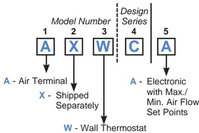
A Carnes Electronic Thermostat **must be ordered** with the ET Electronic Control Option.
