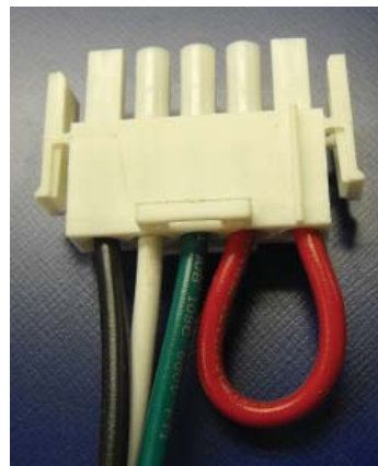
Illustration E - High Voltage Connector for 1/3, 1/2, 3/4 and 1 HP Motors - With Red Jumper Intact for 120-Volt Use
