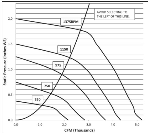
Performance certified is for installation type A - free inlet, free outlet.
